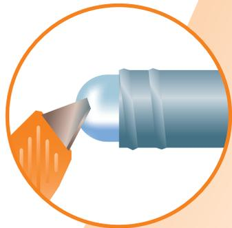
**D Cut or puncture the visible end of cartridge in the barrel.**
