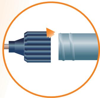
**B Unscrew and remove delivery tube end of the Dryzone application gun.**
