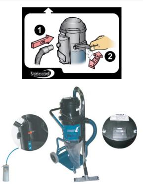
The plastic sack should be changed only after filter cleaning is done and when the collected material level is about 5 cm under the foot valve.
